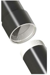
The threaded cylinder joint is available 12" through 16" cylinder diameters. The female threaded coupling is welded to the upper side of the next joint. The cylinder opposite section is threaded to screw into coupling where it is then welded in the field.
