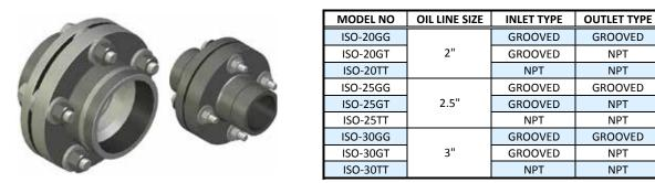
The Isolation Couplings (ISO) are available in three sizes both grooved and threaded. These couplings are designed for electrical isolation with a Dielectric Strength of 42 kV and will also help in the reduction of vibration and noise from being transmitted to the cab. The maximum operating temperature for these Isolation Couplings is 225° F (107° C).
