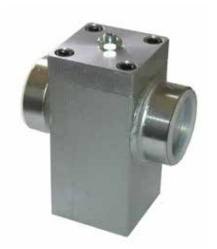
The **Pipe Rupture Valve** (**PRV**) is a simple but effective way to achieve a quick and smooth stopping of a car if an overspeed of the elevator should occur. The PRV is connected directly to the pressure line between the control valve and the jack. The supplied connections on the PRV make installation quick and easy. The PRV comes with either NPT or grooved connections. See table below for Sizes and gpm ranges available.
